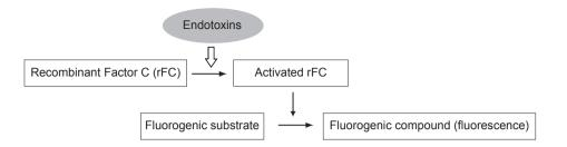
Figure 3. The recombinant Factor C mechanism of reaction [20, 68, 89, 90].
