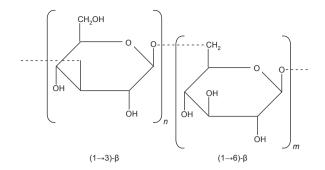
**Figure 4.** Schematic structure of  $\beta$ -glucans [185]. n – number of glucose subunits connected by intrachain glycosidic  $(1\rightarrow 3)$ - $\beta$ -linkages; m – number of glucose subunits connected by intrachain glycosidic  $(1\rightarrow 6)$ - $\beta$ -linkages.
